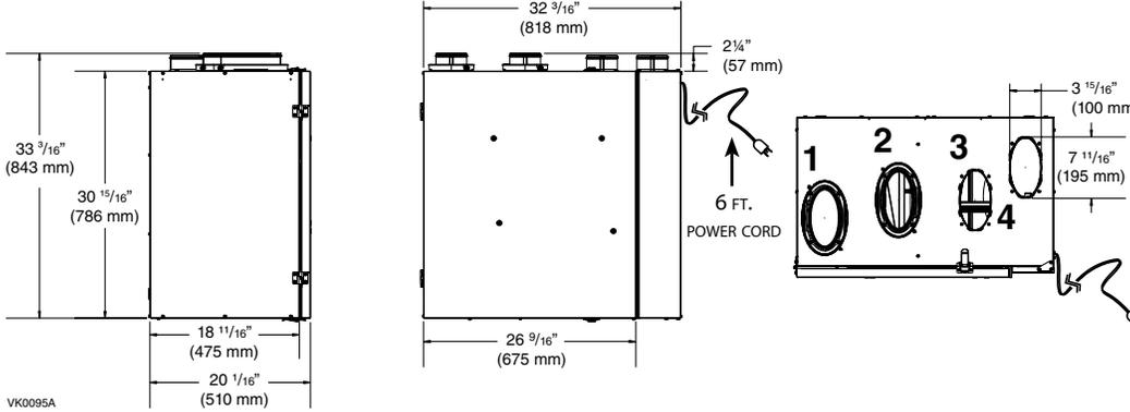
NOTE: ALL UNITS PORTS WERE CREATED TO BE CONNECTED TO DUCTS HAVING A MINIMUM OF 6" DIAMETER, BUT IF NEEDED, THEY CAN BE CONNECTED TO BIGGER SIZED DUCTS BY USING AN APPROPRIATE TRANSITION (E.G.: 6" DIAMETER TO 7" DIAMETER TRANSITION).
