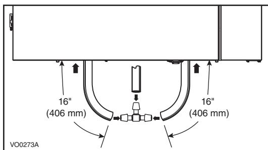
Cut 2 sections of the plastic tube, at least 16" long, and attach them to each inner drain fitting, located under the unit.
