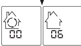
LCD screen alternates between the house with circled arrows and the house without arrow. The numbers under the house are the software version number.
