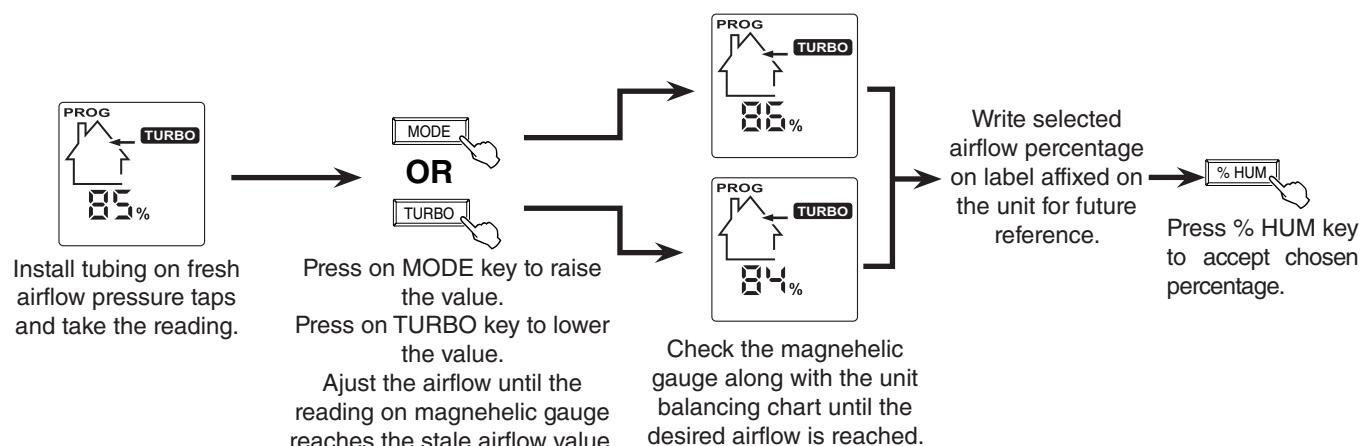
If you have selected the preset speed balancing at ⑦, the balancing procedure is completed.
