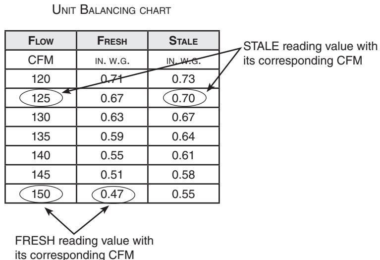
NOTE: The unit is considered balanced even if there is a difference of  $\pm 10$  CFM (or  $\pm 5$  L/s or  $17$  m<sup>3</sup>/h) between the two airflows.
