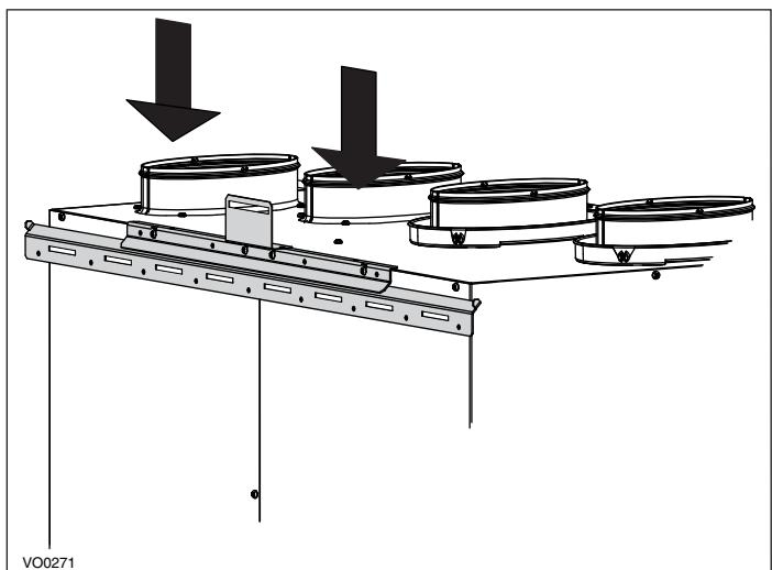
Secure the unit to the wall using one 1½" long provided screw through the small bracket.
