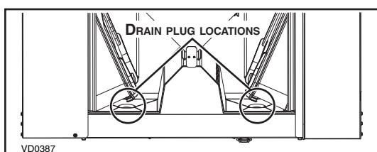
NOTE: For ERV units installed in cold climate, remove both drain plugs inside the unit prior to install tubing.
