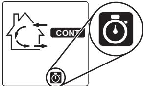
When used, the VB60W activation will override the main control operation, as well as the unit defrost cycle. On example shown on the left, the unit was in CONT mode when the auxiliary control was activated; so the actual operation mode stays on VT9W main wall control screen, but the chronometer icon appears as long as the VB60W is activated.
