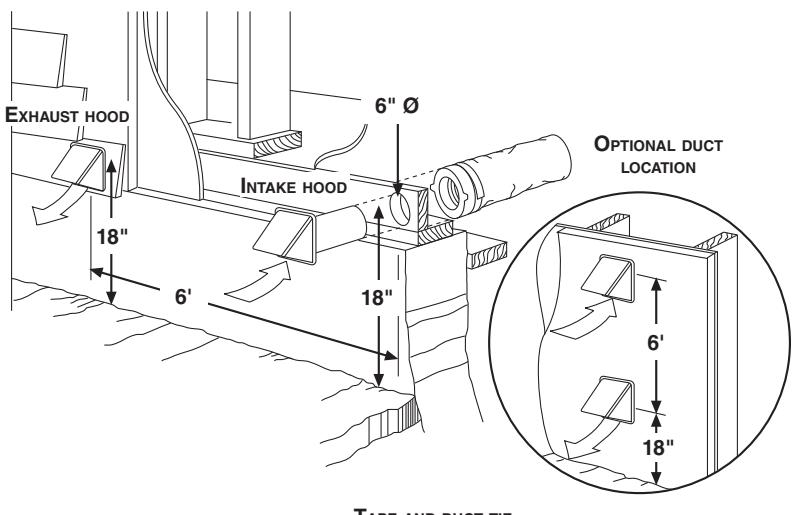
Refer to figure at right for connecting insulated ducts to the exterior hoods. An "Anti-gust intake hood" should be installed in regions where a lot of snow is expected to fall.
