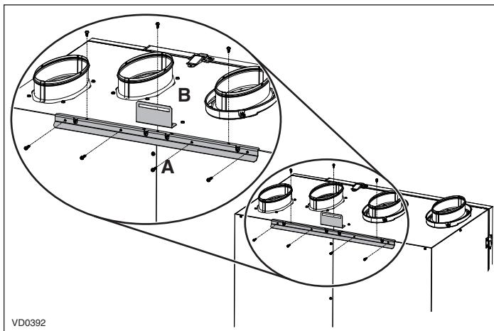
Lift the unit and hang it to the wall bracket. Ensure the bracket assembled on back of the unit rests on the wall bracket.
