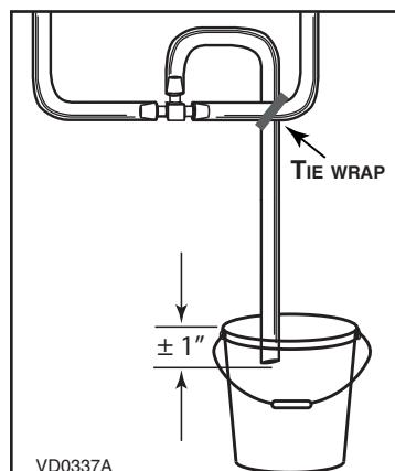
Make a water trap loop in the tube to prevent the unit from drawing unpleasant odors from the drain source. Make sure this loop is located OVER the "T" as shown. Run the tube to the floor drain or to an alternative drain pipe or pail.
