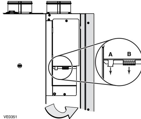
Run the end of the control wire(s) through the grommet located on the unit wall. Refer to illustration at right (side panel removed to ease understanding).
