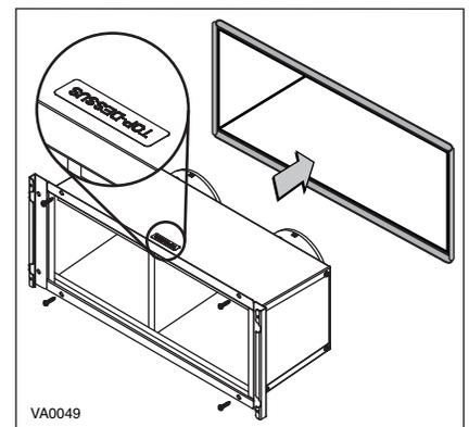
ASSEMBLE THE GRILLE TO THE METAL TANDEM HOOD BOX USING BOTH N° 8 x 3/8" SCREWS PREVIOUSLY REMOVED PLUS 2 OTHER N° 8 x 3/8" SCREWS FROM PARTS BAG. SEAL THE OUTLINE WITH CAULKING.
