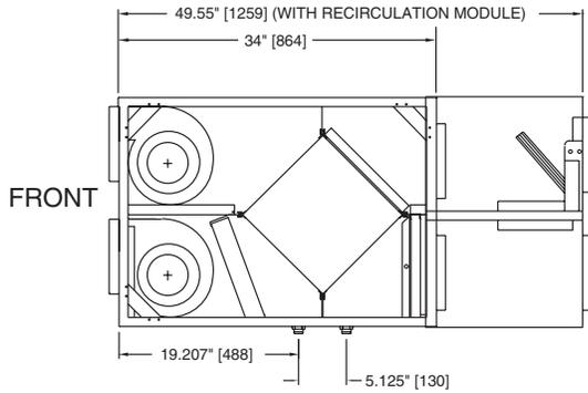
A MINIMUM OF 12" [305] CLEARANCE FROM ANY OBSTRUCTION IS REQUIRED FOR REMOVAL OF CONTROL BOX.
