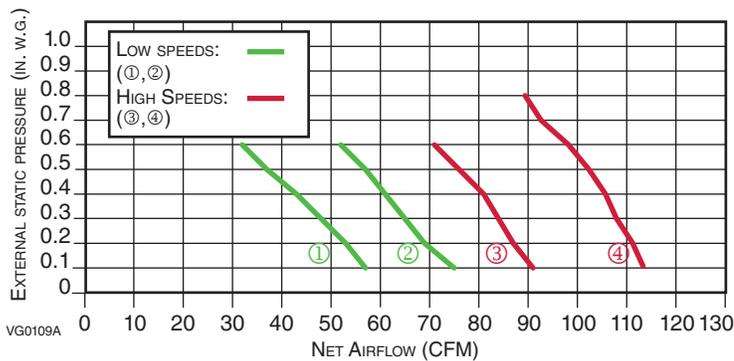
NOTE: Low speed ① and high speed ④ are factory set, low speed ② and high speed ③ are selectable.
